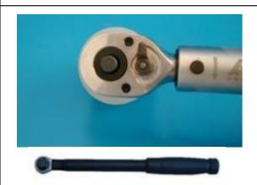
9. Take the torque wrench and set the indicator to the "close" position.
