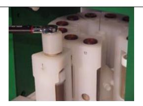
17. Tighten the reference vessel in the same way as the other vessels.
