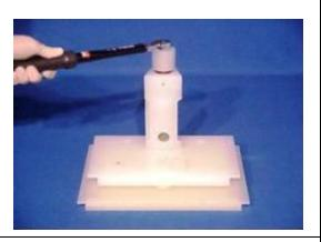
29. Place the work station under a fume hood, and carefully loosen the screw in the upper part of each individual segment, by using the torque wrench.
