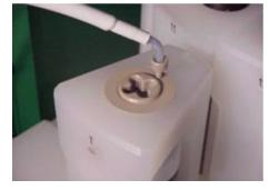
Fully introduce the temperature sensor into the thermowell, until the snap connector is fixed.
