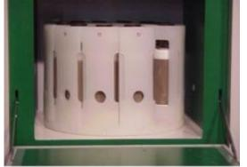
13. Reference vessel must be used as a standard vessel, therefore the same acid volume/mixture and the same sample type/amount must be placed into it.
