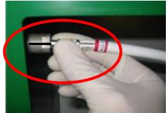
Plug-in and unplug the temperature sensor, again touching only the metal plug.
