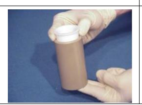
33. Slide the TFM Teflon vessel out of the HTC protection shield.
