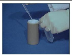
3. Add suitable reagents to the sample. When part of the sample is left on the inner wall, try to wet it by adding acids drop by drop.
