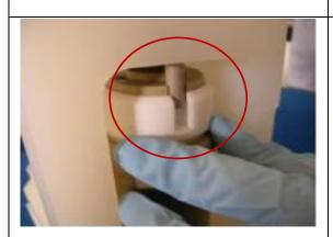
16. Introduce the reference vessel just assembled into the reference polypropylene segment.
