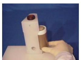
30. Remove the vessel from the polypropylene segment.
