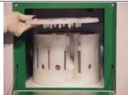
20. Introduce the segmented rotor top plate; the plate is fixed by the connectors to each individual polypropylene segment.
