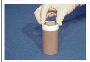
7. Place the TFM Teflon indicator ring on the cover and push it down completely.
