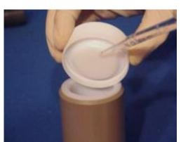
32. Rinse the lower part of the TFM Teflon cover with distilled water, collecting the same inside the vessel.
