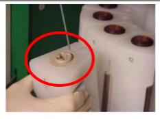
Introduce the thermocouple into the reference vessel, simply sliding-in the sensor through the hole in the HTC screw of the reference segment.
