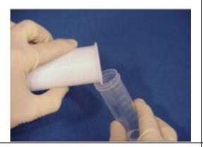
34. Pour the solution in a laboratory volumetric flask, washing repeatedly the TFM Teflon vessel with distilled water.
