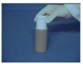
2. Introduce the Teflon vessel into the HTC protection shield.
