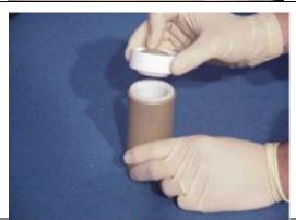
31. Carefully lift up the vessel cover, together with the TFM Teflon indicator ring.
