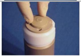
15. Put the special HTC adapter plate and safety spring. The reference HTC spring differs from the others; it has a smaller diameter to allow the introduction of the thermocouple into the vessel.
