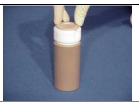
14. The special HTC adapter plate goes onto the reference TFM Teflon cover.
